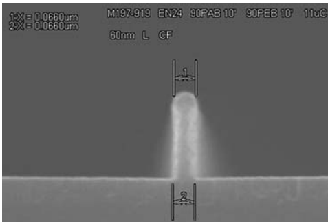
Figure 3.57 A negative CAR EN24 (TOK) showing 60-nm resolution. (Courtesy R. Dean.)
