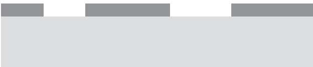
Figure 8.7 Schematic cross sections illustrate the mask fabrication steps required to build a subtractive-ML EUVL mask.
