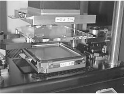
Figure 6.38 Semiautomated pellicle mounter. (Source: Cotte, E. P., R. L. Engelstad, E. G. Lovell, F. Eschbach, D. Tanzil, "Effects of soft pellicle frame curvature and mounting process on pellicle-induced distortions in advanced photomasks," Proc. SPIE 5040, pp. 1044–1054, 2003.)
